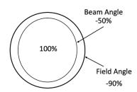
Beam Angle: Light beam is no less than 50% of the brightest part of the light beam.
